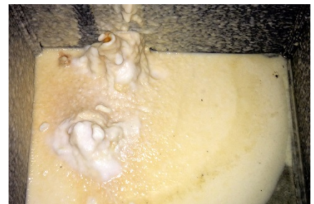
Produced water solids
