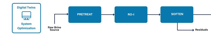
Process Step Pre-conditioning System (PCS) Primary Reverse Osmosis Scaling Ion Removal
