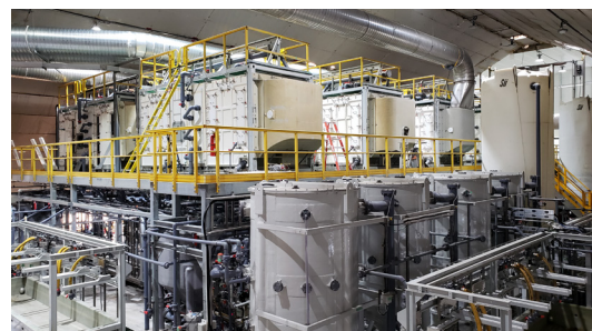
SaltMaker plant treating mine water at client site
