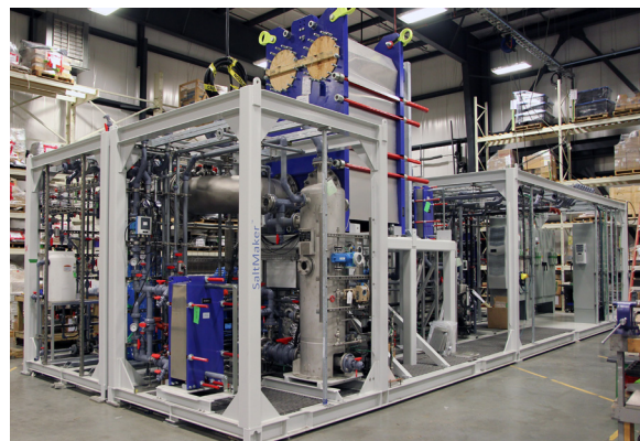
A SaltMaker MVR plant being assembled
