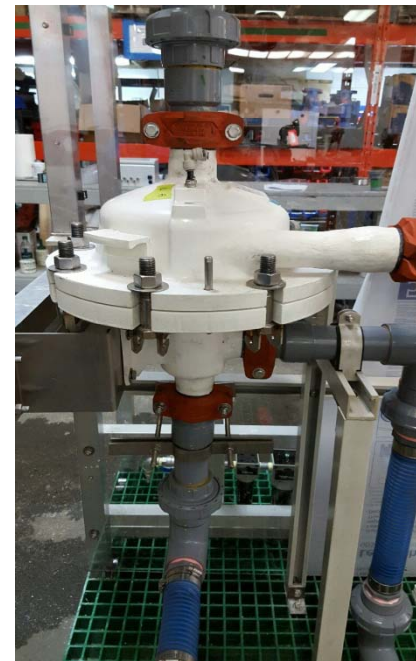
50 \mu m self cleaning filter for > 50 \mu m solids
