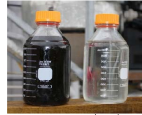
Raw blowdown (left) and SaltMaker condensed water (right)
