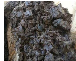
SaltMaker solids suitable for Class II landfill disposal
