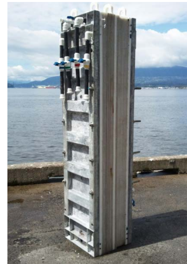
Saltworks' micro EDR stack (left) and full scale EDR stack (right)
