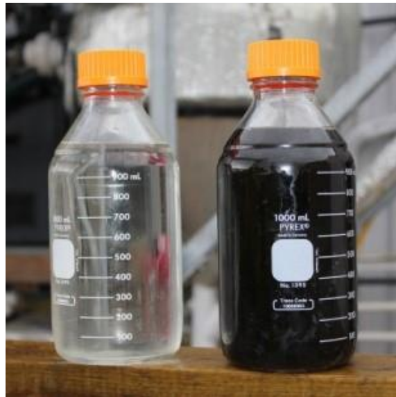
Raw blowdown (left) and SaltMaker condensed water (right)
