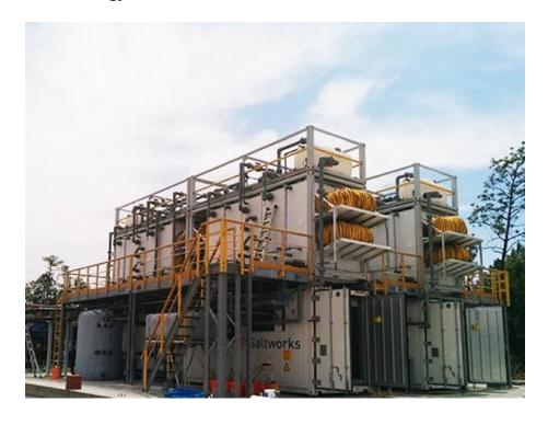
When considering a closed evaporative crystallizer, you should also factor pre-treatment for scaling, concentration limits of conventional evaporators, and corrosion risk. In addition, if freshwater is produced, it must either be stored, re-used, or released to the environment. One advantage of freshwater storage and transportation over produced water storage is that it requires less containment. Although you should check your local regulations,
