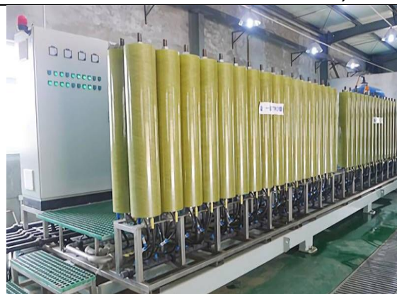
Figure 3: DTRO membranes (radial flow over membrane disks)
