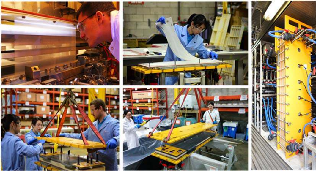
Figure 4: Full Scale Production of Electrodialysis Stacks and Membrane 图4：大规模电渗析膜堆和膜生产
