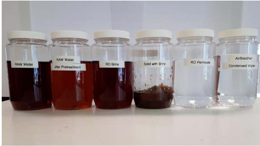
Figure 2: (1) Raw Water, (2) After BrineRefine, (3) XRO Brine, (4) AirBreather Solid, (5) XRO permeate and (6) AirBreather Condensed Water (From left to right)
